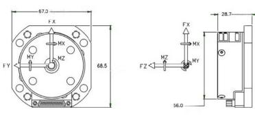
Fig. 2: Dimensions in mm
