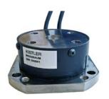
In order to avoid linearity errors, the deformation paths are constructively held small (high stiffness); thus a proportional behavior is realized. The force and moment proportional resistance variations are measured by a Wheatstone-type bridge circuit.
