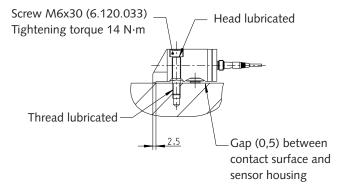
Fig. 5: Mounting with 6-point socket head cap screw
