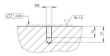
Fig. 3: Preparing the mounting surface
