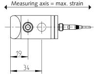
Fig. 4: Aligning sensor to the strain axis
