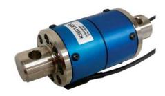
In order to avoid linearities, the deformation paths are constructively held small (high stiffness). Thus a proportional behavior is realized. The force and moment proportional resistance variations are measured by a Wheatstone-type bridge circuit.
