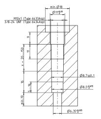
Fig. 2a: Bore for mounting with mounting sleeve
