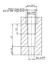
Fig. 1a: Bore for direct mounting
