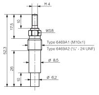
Fig. 7: Dummy sensor Type 6469A1 (M10x1) Dummy sensor Type 6469A2 ( $^3/_8$ " – 24 UNF)
