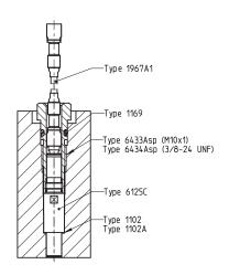
Fig. 2: Mounting sensor Type 6125C... with mounting sleeve
