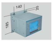
Wall mounted housing with fixing hole
