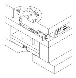
Fig. 4: Sensor, cable, mounting plate and identification plate
