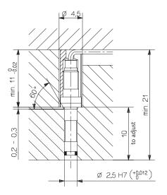
Fig. 3: Installation with spacer sleeve Type 6464
