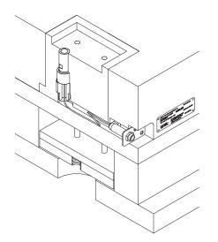
Fig. 3: Sensor, cable, mounting plate (Art. No. 3.520.328) and identification label (Art. No. 3.520.842)
