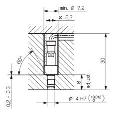
Fig. 2: Installation with spacer sleeve (Type 6459)
