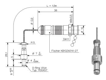
Alternative version of sensor Type 6167A... with single-wire technique. Simplified sensor installation thanks to the single-wire cable, which can be flexibly installed in the mold and cut to length as required. Both single-wire cable and connector are exchangeable.
