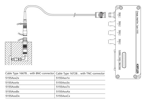
Fig. 2: Sensor Type 6167A... with charge amplifier Type 5155A... (1-, 2- or 4-channel; SmartAmp optional on one channel)
