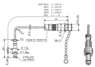
Quartz sensor for mold cavity pressures up to 200 bar for processing low-viscosity plastic melts (e.g. sheaths of IC components). Exchangeable high-temperature cable with connector.
