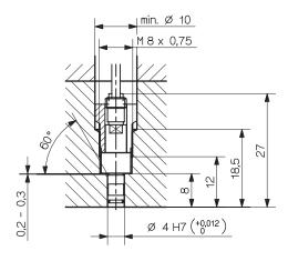
Fig. 1: Installation with mounting nut (Type 6457)
