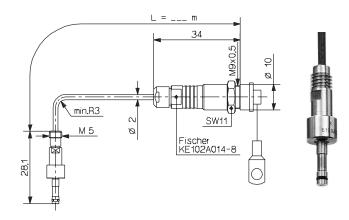
Fig. 1: Quartz sensor for mold cavity pressures up to 2 000 bar for the injection molding of plastics.
