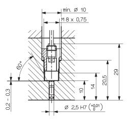
Fig. 5: Installation with mounting nut Type 6457
