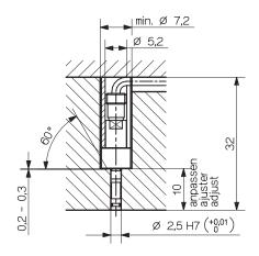
Fig. 6: Installation with spacer sleeve Type 6459
