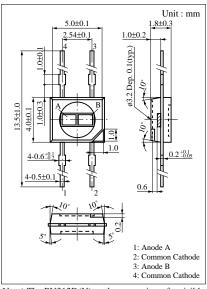
Note) The PN312D(N) package consists of a visible light cutoff resin. Therefore the chips (A and B) shown in the drawing cannot actually be seen.
