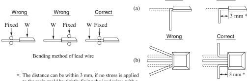
\*: The distance can be within 3 mm, if no stress is applied to the resin mold by tightly fixing the lead wires with a metallic mold or the like.
