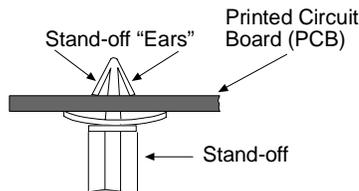
Be sure that the Stand-off is pressed firmly through the Printed Circuit Board, so that the Stand-off ears can expand outward.
