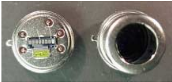
Figure 7b: Thermopile line array with ASIC containing the multiplexer and amplifier. The right side shows the capped sensor with micromachined silicon lens.
