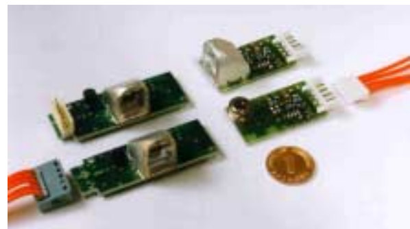
Figure 9: PerkinElmer Optoelectronics thermopile modules with mirror optics. The modules have an on-board signal amplification and temperature compensation and come completely calibrated – ready to plug-in. The employed system guarantees full interchangeability, which makes a manufacturing process easy. In case of service requirement, one can simply replace one module by another.
