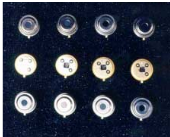
Figure 6: Thermopile sensors: The upper and the lower rows are sensors in TO housings sealed under inert atmosphere. The round hole is the infrared window, through which the radiation reaches the absorber.
